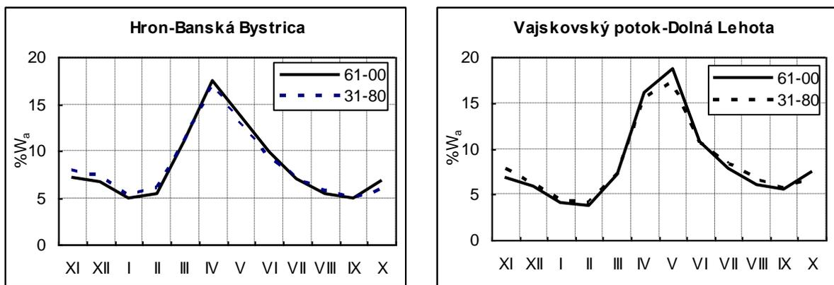
Figure 6. Comparison of mean monthly runoff for the periods 1931-80 and 1961-2000 for two selected subcatchments of the Hron catchment (Pekarova and Szolgay, 2005).
