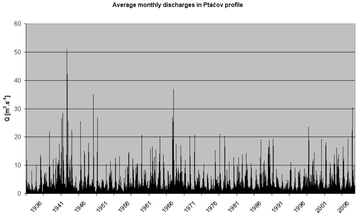
Figure 11. The average monthly discharges in Ptáčov profile (catchment area 960 km<sup>2</sup>).
