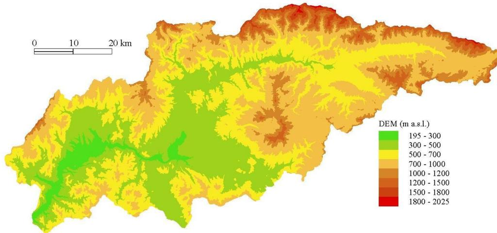
Figure 2. Digital elevation model (DEM) of the Hron River basin (50x50 m resolution)
