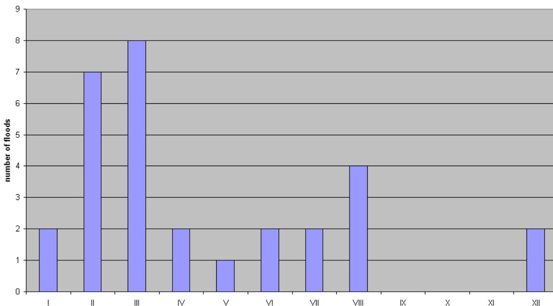
Figure 9. The occurrence of floods with peak discharge greater than  $130 \text{ m}^3 \cdot \text{s}^{-1}$  in Podhradi profile. It is obvious that winter floods caused by snowmelting are the most common in this catchment, the summer floods occurred most frequently in August. The measurement in the Podhradi gaugestation started in 1934.
