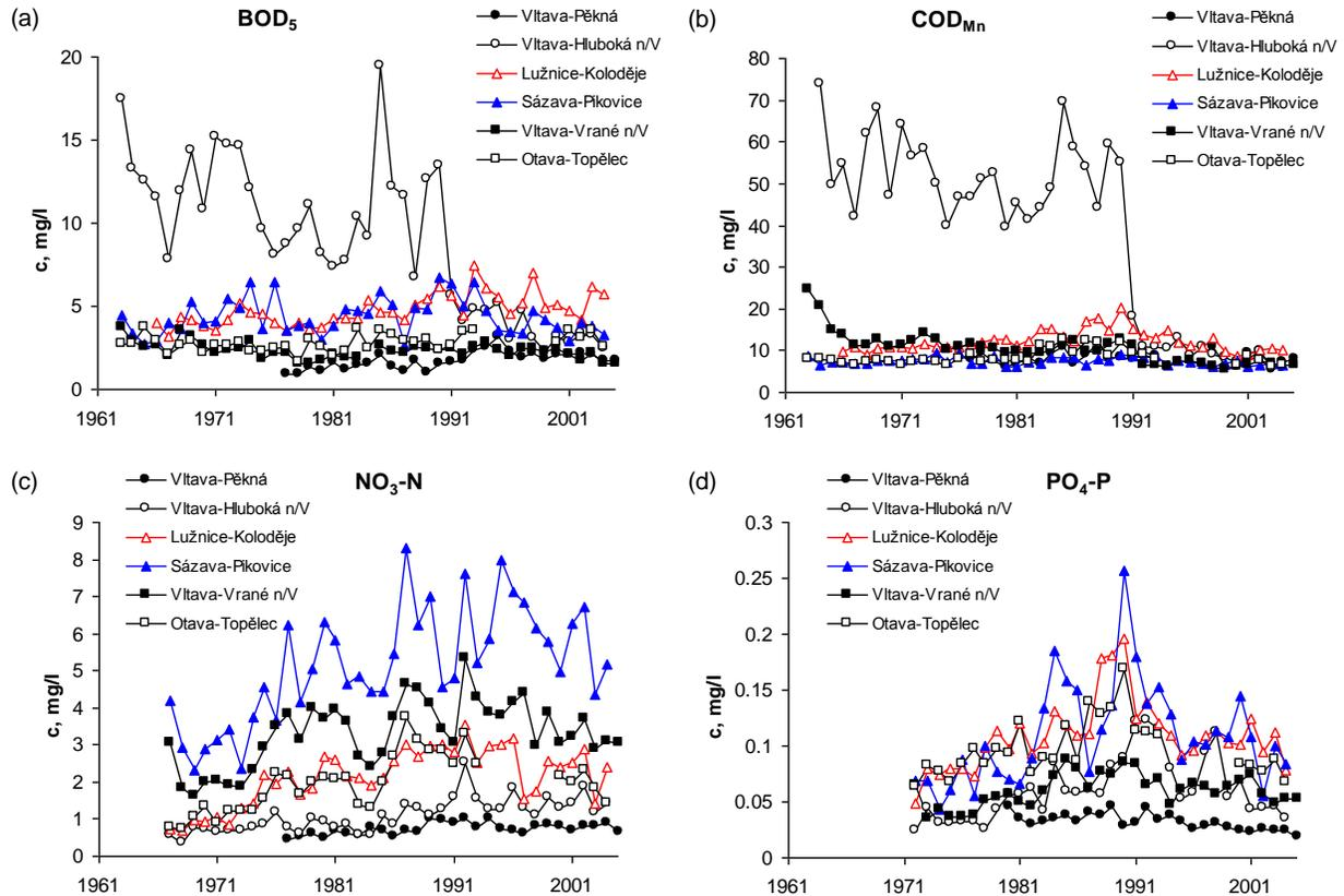
Figure 2. The time series of annual mean concentrations of (a)  $BOD_5$ , (b)  $COD_{Mn}$ , (c)  $NO_3-N$ , and (d)  $PO_4-P$  in selected monitoring stations in the upper Vltava River basin (see Figure 1 for their location) during available data periods
