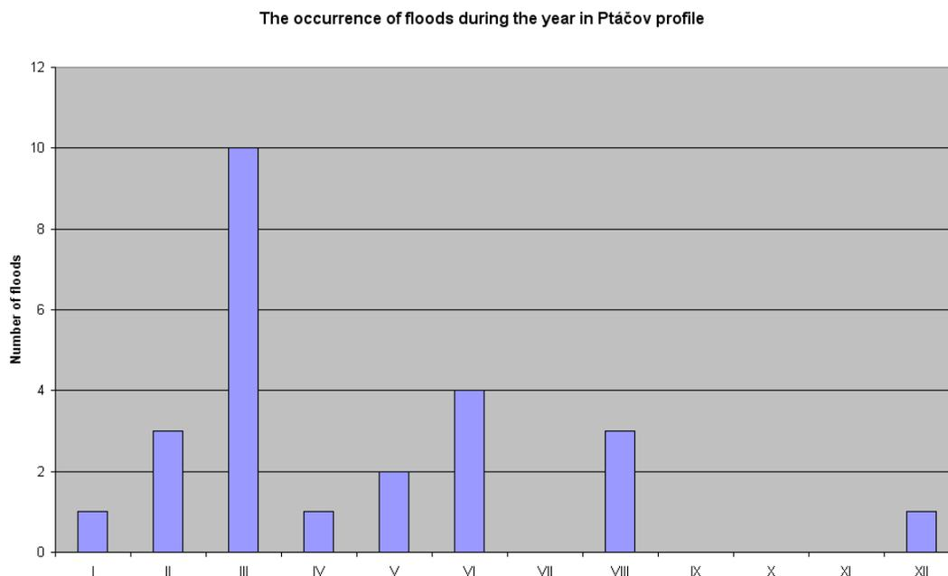
Figure 13. The occurrence of floods with peak discharge greater than  $70 \text{ m}^3 \cdot \text{s}^{-1}$  in Ptáčov profile. Again, the winter floods caused by snowmelting are the most common. The measurement in the Ptáčov gaugestation started in 1932.
