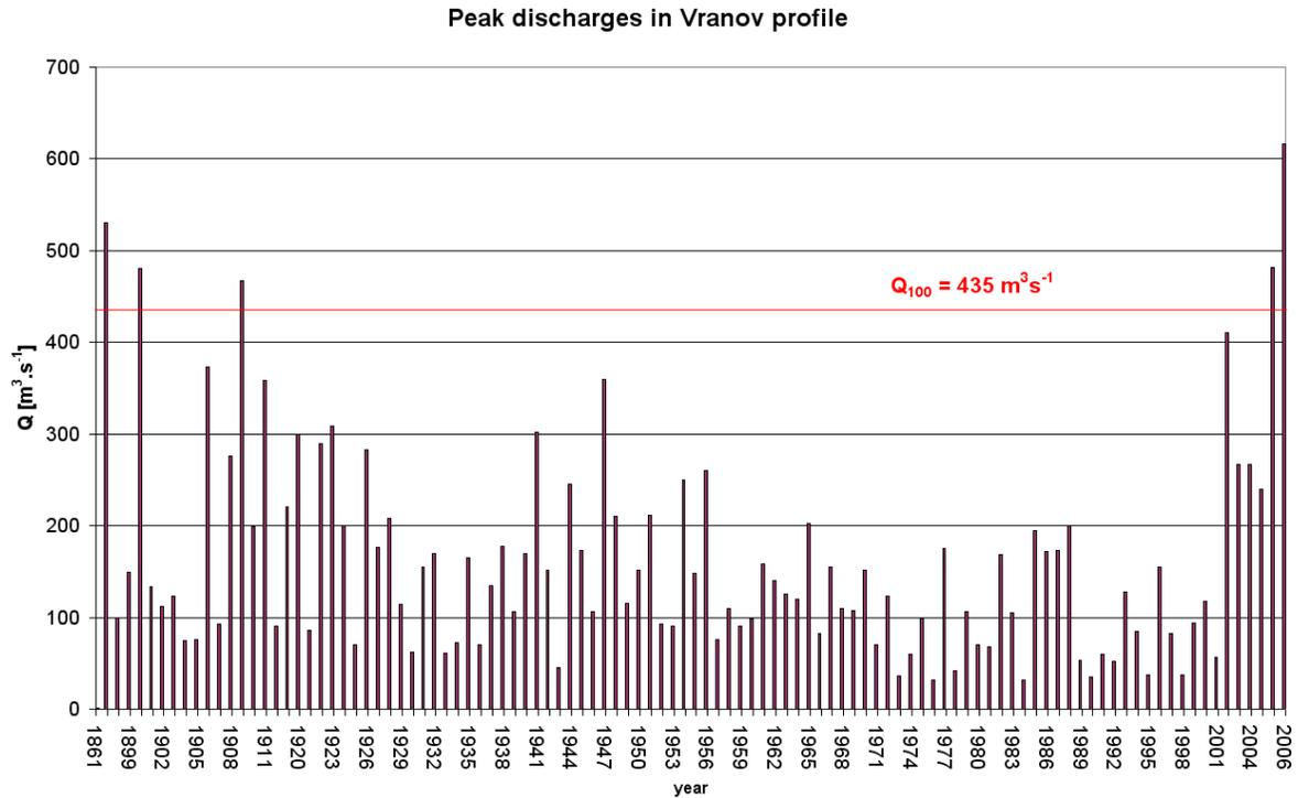
Figure 4. The graph of annual maxima discharges in Vranov profile (the dam of Vranov reservoir, 20 km downstream from the Podhradí station). In the last 5 years three huge floods occurred, while the record culmination was reached in July 2006.
