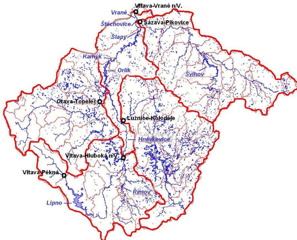
*Figure 1. The upper Vltava River basin with major rivers and reservoirs. Circles – selected hydrology and water quality monitoring stations; thick red line – the main catchments described in text; little red line – the subcatchments used in HSPF modelling.*
