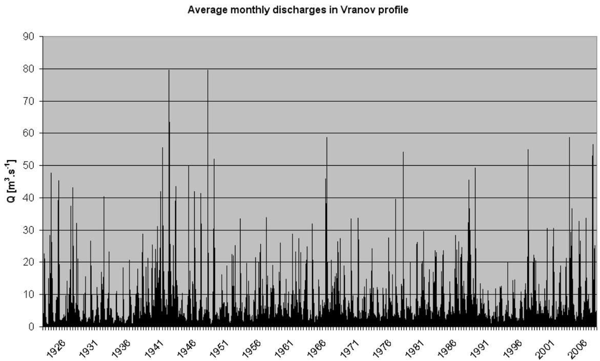
Figure 6. The average monthly discharges in Vranov profile (catchment area  $2220\text{ km}^2$ ).
